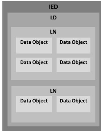
Figure 5: Data Structure in IEC 61850
